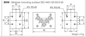
For versions 11 and 13 the pressure switch is mounted on side of port A. For version 14 the pressure switch is mounted on side of port B. For versions 12, 17, 18 the pressure switch is mounted on both sides.
