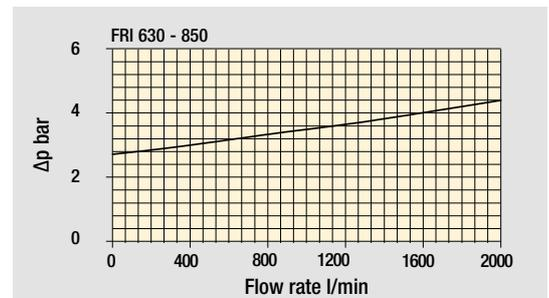
The curves are plotted using mineral oil with density of  $0.86 \text{ kg/dm}^3$  in compliance with ISO 3968.  $\Delta p$  varies proportionally with density.
