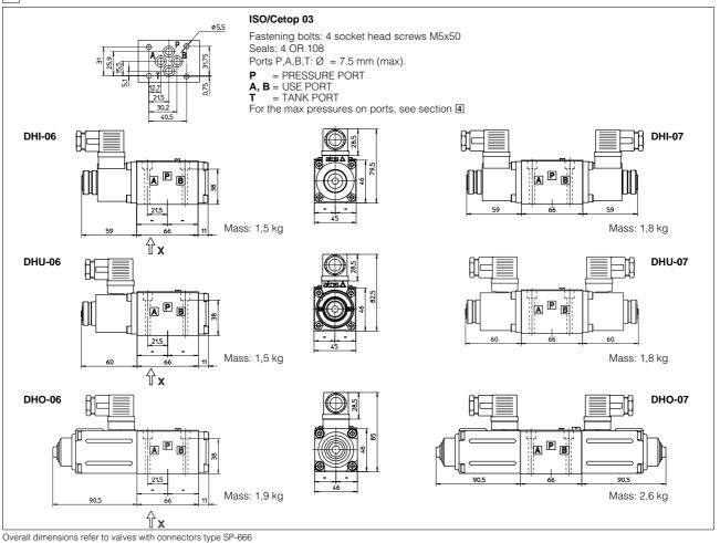
11 ELECTRIC/ELECTRONIC CONNECTORS ACCORDING TO DIN 43650 - The connectors must be ordered separately
