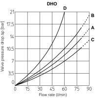
Based on fluid viscosity of 43 mm²/s at 40°C
