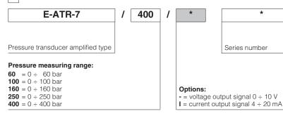
E-ATR-7 pressure transducers measure the static and dynamic pressure of the hydraulic fluid, supplying a voltage or current output signal.
